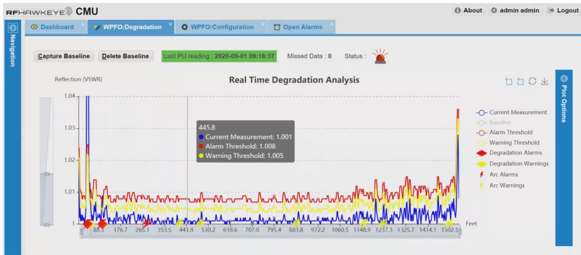
RFH Degradation Plot Showing Transient Response Disappearance and Degradation Alarm Active
