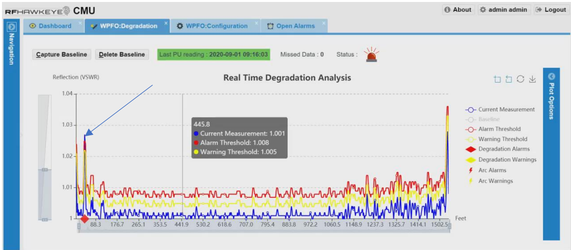
RFH Degradation Plot Showing Degradation Alarm Status as Measurement Exceeds Alarm Threshold
