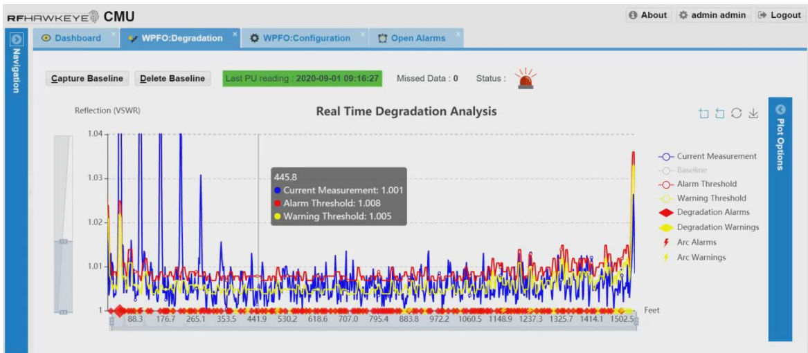
RFH Degradation Plot at instant of Arc Occurrence and Transient Response Beyond the Arc
