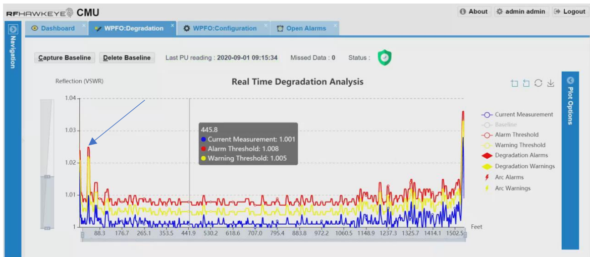
RFH Degradation Plot Under Normal Operation with Current Measurement , Warning Threshold , and Alarm Threshold Traces. Arrow Indicates Location of Probe Insertion.
