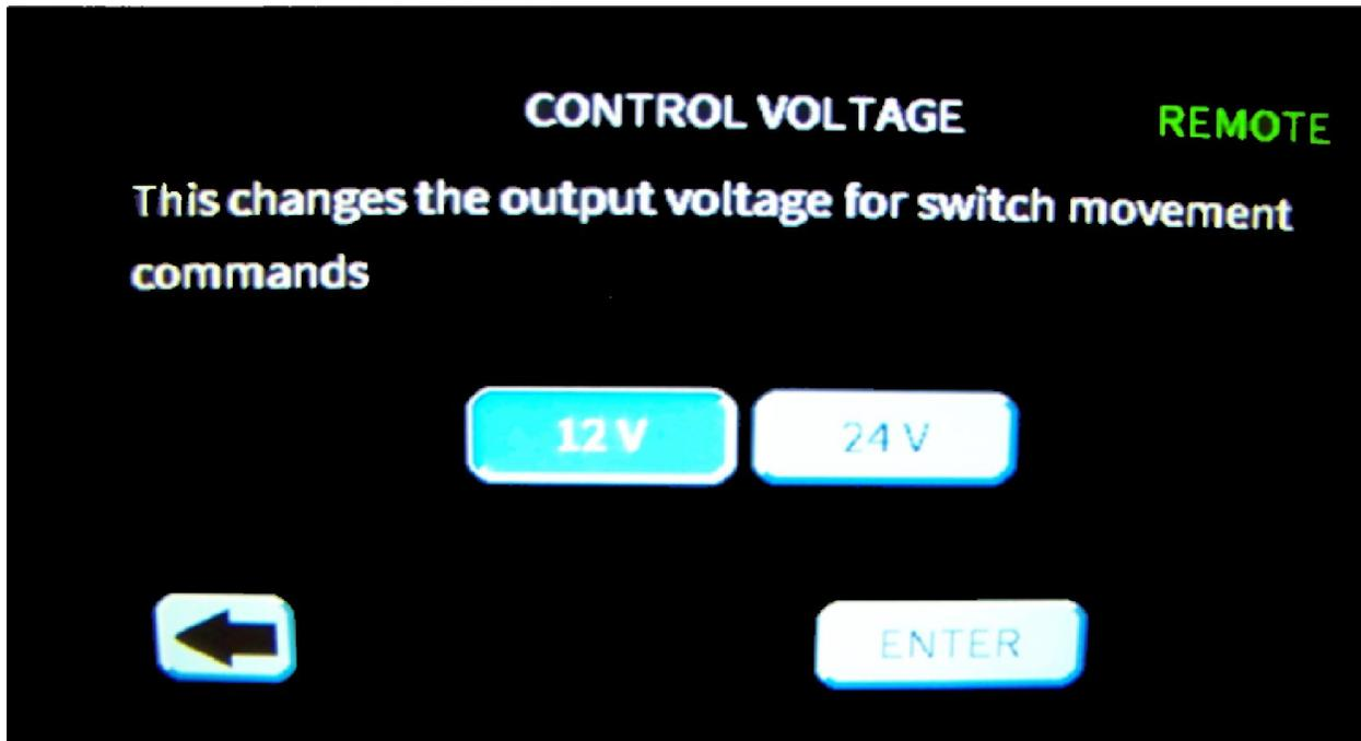
Figure 3: Voltage configuration
