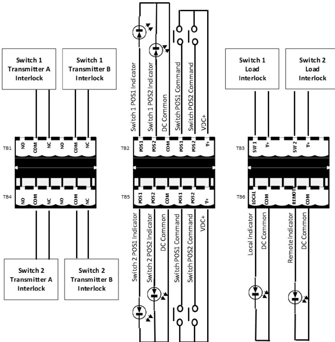
Figure 7: Pinouts on rear panel of the Dual Switch Controller
