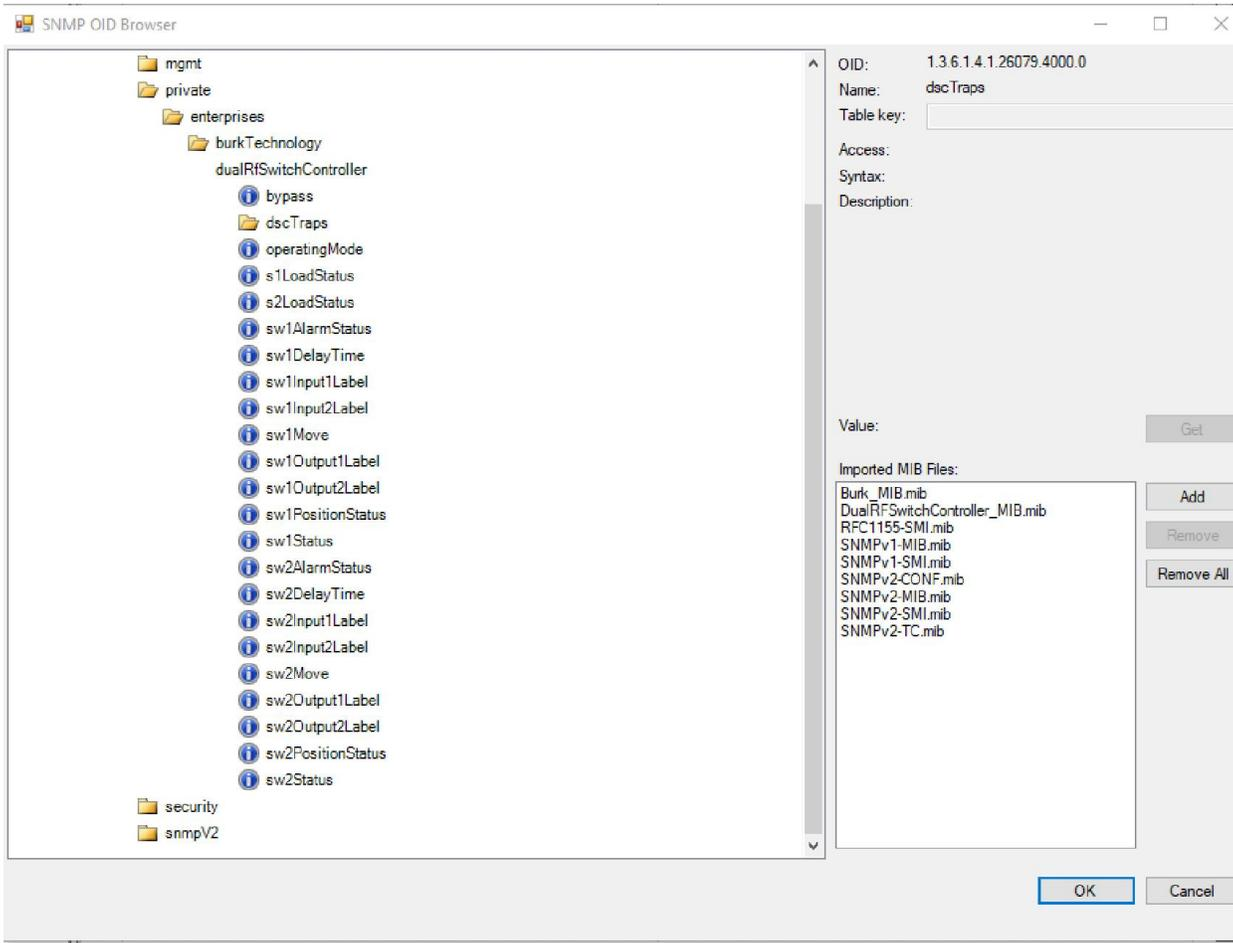
Figure 21: SNMP mib file browser showing list of SNMP functions
