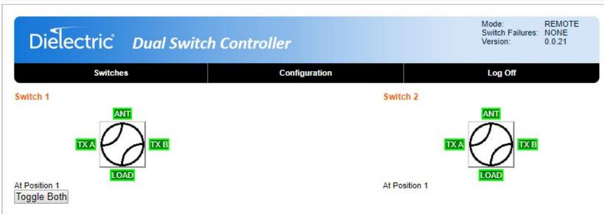
Figure 20: Switch position display using web interface
