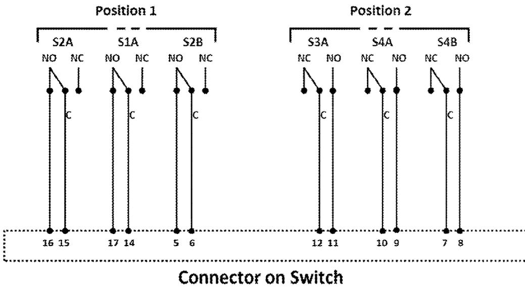
Figure 9: Limit switch configuration and pinout in RF Switch
