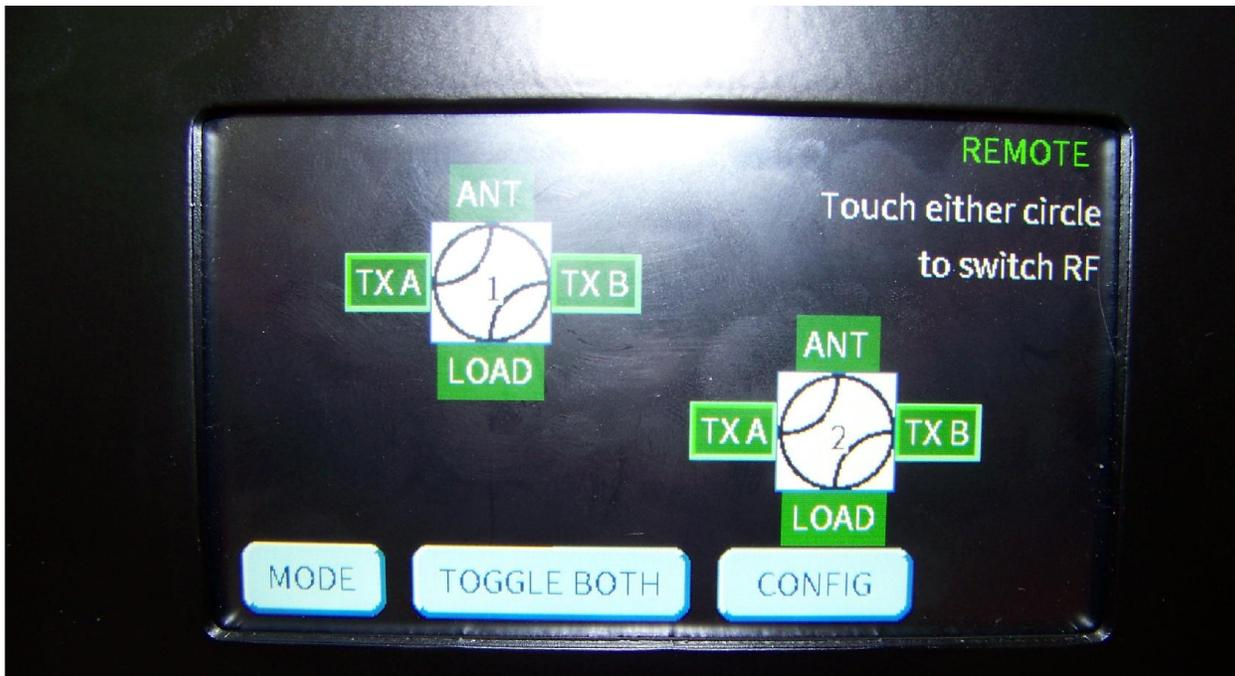
Figure 11: Dual switch controller monitoring RF switch position
