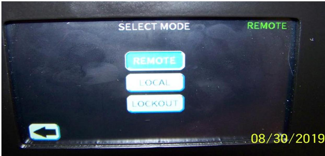
Figure 12: Dual Switch Controller modes of operation
