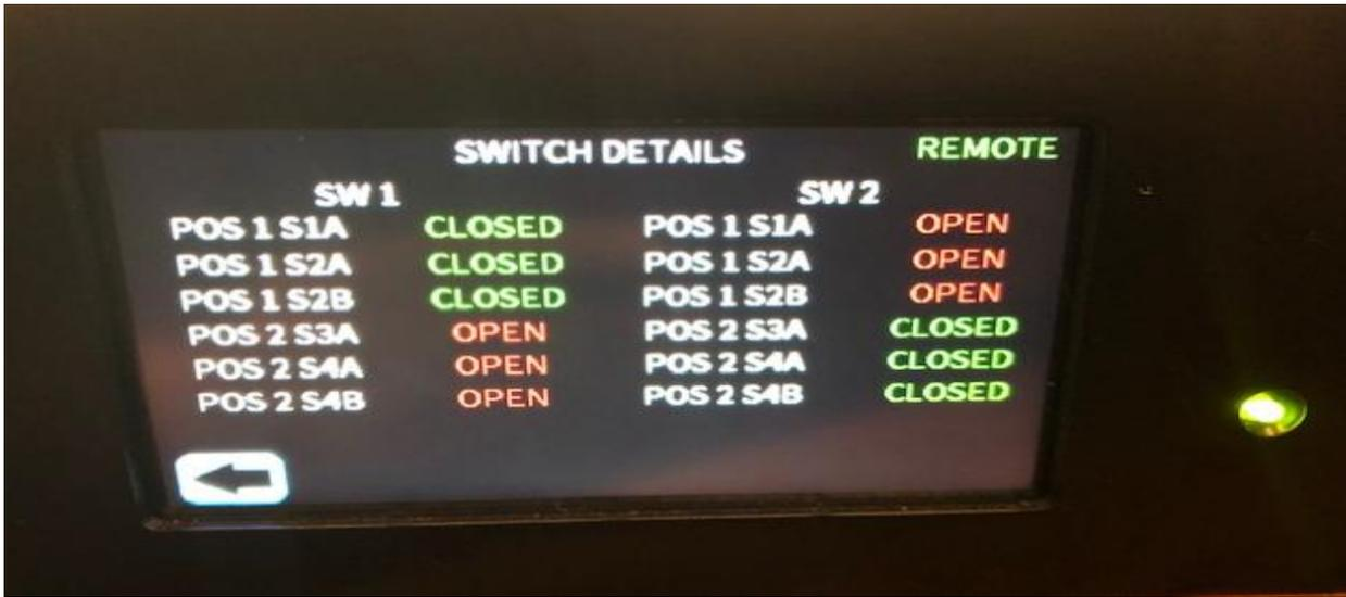
Figure 10: Switch position details
