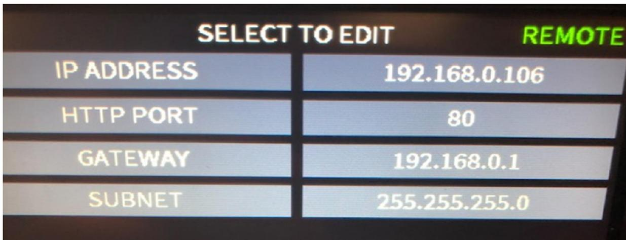
Figure 2: IP Address Configuration
