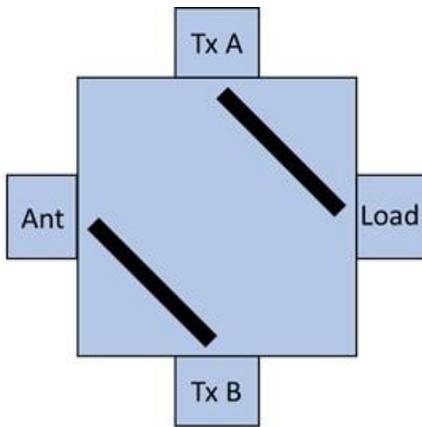
Upon receiving an activation command from the Dual Switch Controller, the RF Switch moves to Position #2 (POS #2). The RF signal flow is:
