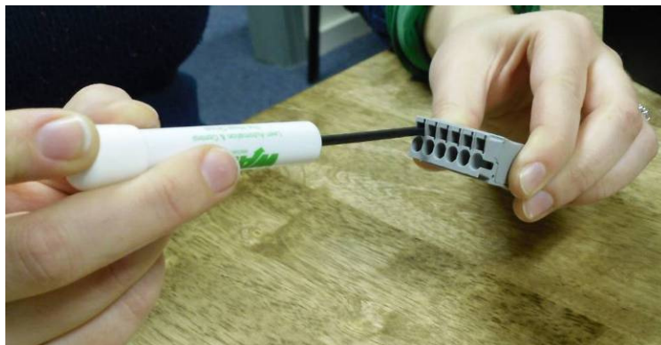
Figure 3.2 - Screw-less connector wire installation
