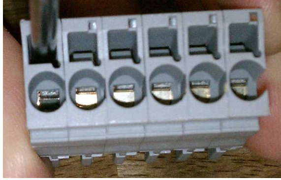
Figure 3.3 - Screw-less connector with open cage
