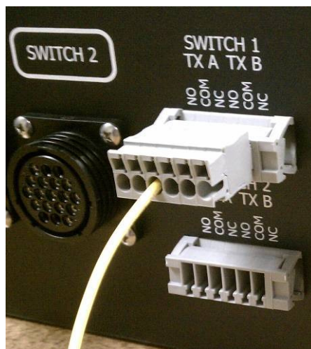
Figure 3.5 - Screw-less connector inserted into Dual Switch Controller
