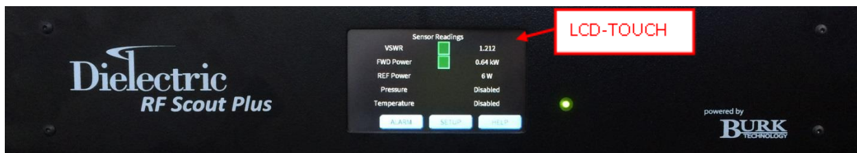
Figure 2.1 – RF Scout Plus Front Panel
