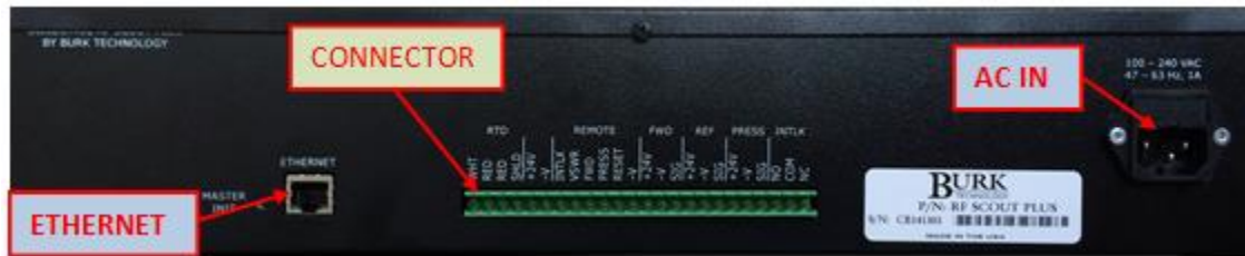
Figure 2.2 – RF Scout Plus Rear Panel
