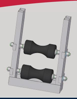
Supports single horizontal line. Two required for dual lines. Mounting bolts not supplied. Rollers accommodate no vertical movement; use 3-point suspension hangers for horizontal runs when length of vertical run or stiffness of line will require vertical as well as horizontal movement of the horizontal run.
