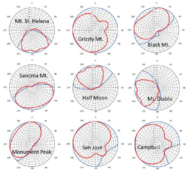
Figure 21: Real WB antenna patterns overlaid on the theoretically generated patterns. Blue – theoretical. Red – real.
