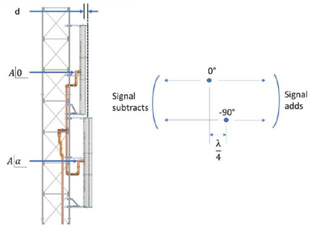
Figure 17: The use of offset WB sections to create a high front to back ratio azimuth pattern.
