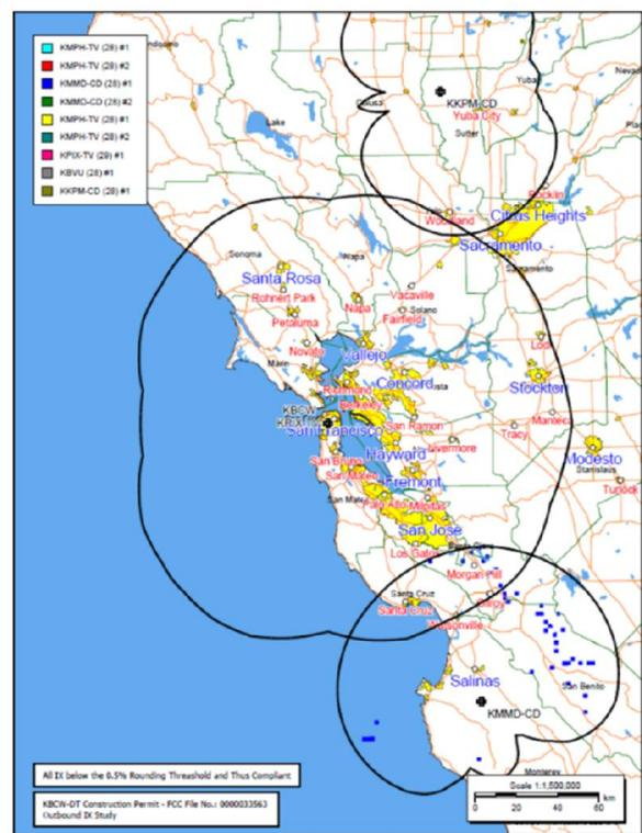
Figure 9: Interference map of KBCW as permitted.
