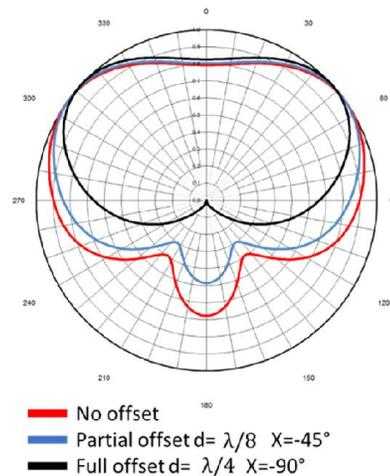
Figure 18: Azimuth patterns of offset WB sections. Varying the offset and feed phase controls the level of front to back ratio.
