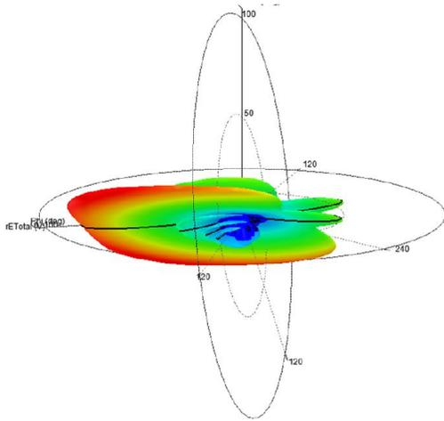
Figure 19: Full 3-dimensional radiation pattern of two 8-layer WB sections using full  $\lambda/4$  offset and 90-degree phasing.
