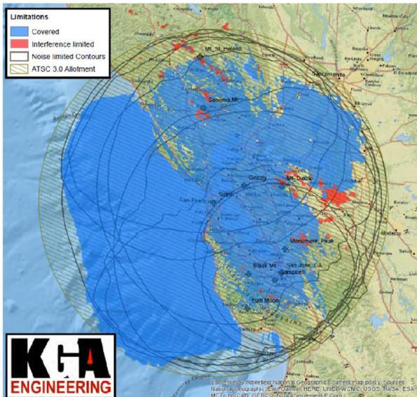
Figure 7: SFN sites after power reductions defining the best fit theoretical patterns.
