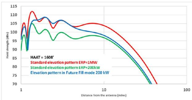
Figure 26: KBCW signal strength vs. distance from the antenna. Comparison of current operation, reduced ERP to meet the contour limit with the addition of an SFN and switching to Future Fill mode with SFN's.
