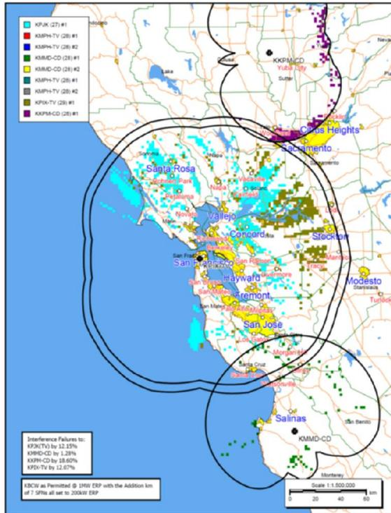
Figure 10: Interference map of KBCW with the addition of the 9 SFN sites.
