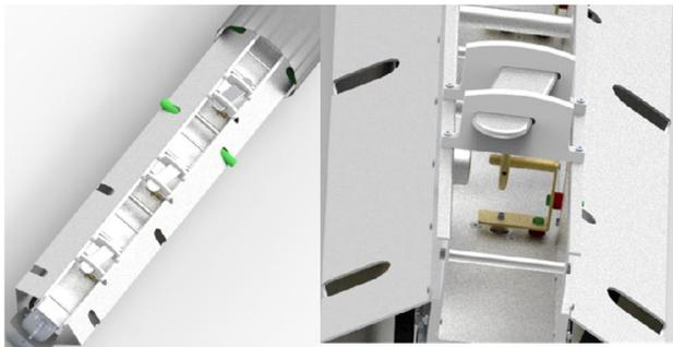
Figure 16: Slot cavity WB antenna.
