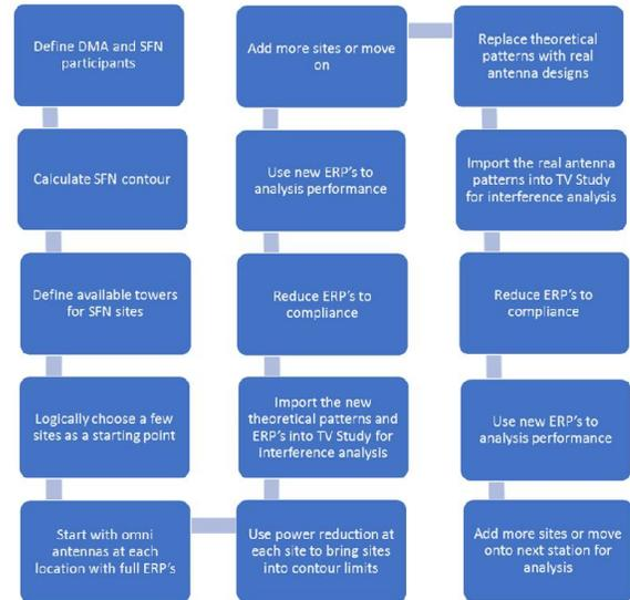
Figure 4: Fundamental flow chart of the SFN design process.
