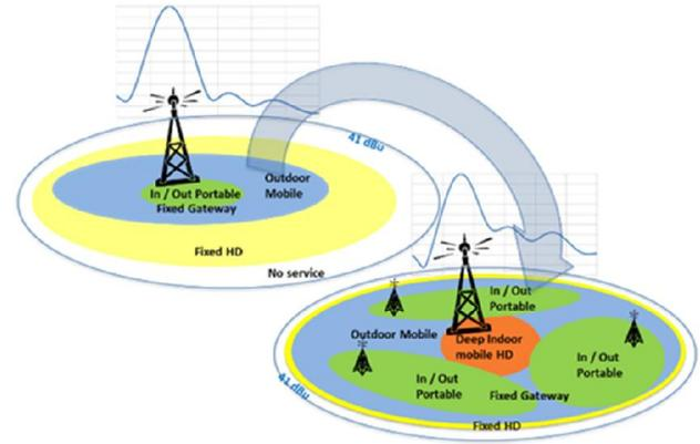
Figure 1: Saturate with main antenna and add SFN sites to boost the service and provide targeted data intensive services.
