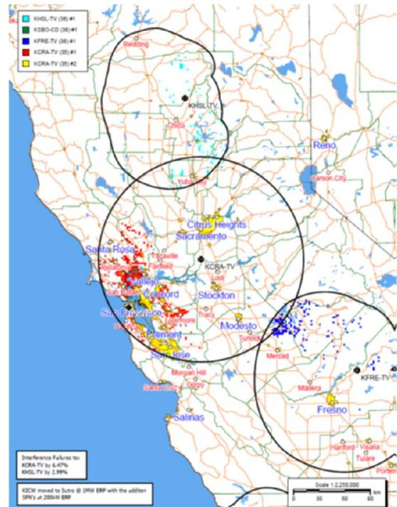
Figure 13: Interference map of KICU with the addition of the 9 SFN sites.
