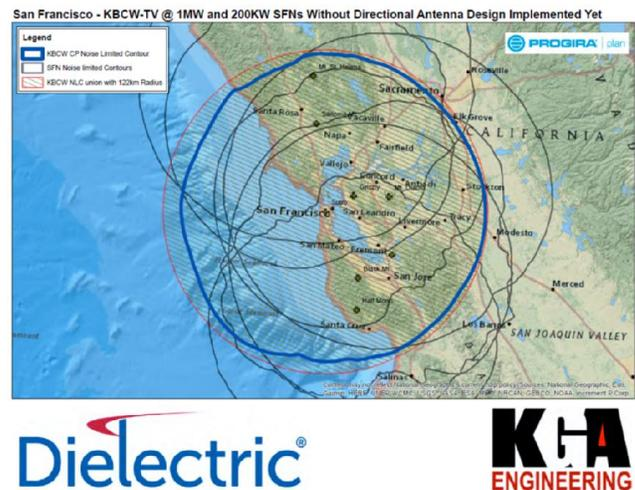
Figure 6: Chosen SFN sites start out omni directional before power reduction optimization.
