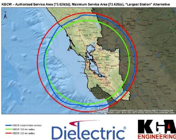
Figure 5: Defining the KBCW service area limits for an SFN in the San Francisco Bay Area based on largest station.
