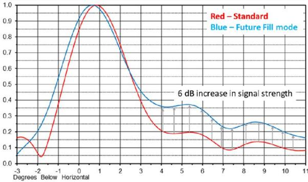
Figure 25: KBCW's standard elevation pattern and Future Fill mode.
