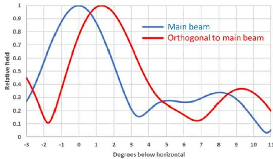
Figure 20: The elevation pattern difference between the direction of offset and orthogonal to the direction of offset.
