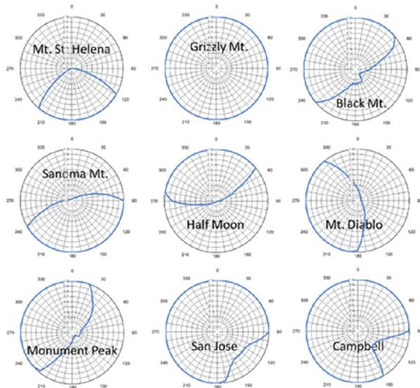
Figure 8: Best fit theoretical azimuth patterns for each site.
