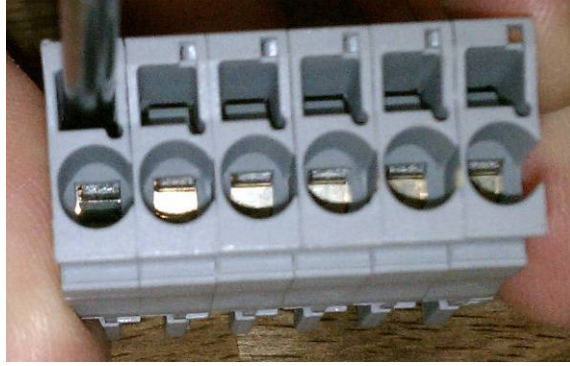
Figure 3.3 - Screw-less connector with open cage
