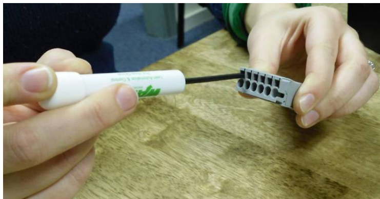
Figure 3.2 - Screw-less connector wire installation
