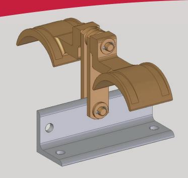
For dual horizontal line runs. Takes care of some horizontal line expansion but permits no vertical movement. Use 3-point suspension hangers for horizontal runs when length of vertical run or stiffness of line will require vertical as well as horizontal movement of the horizontal run.
