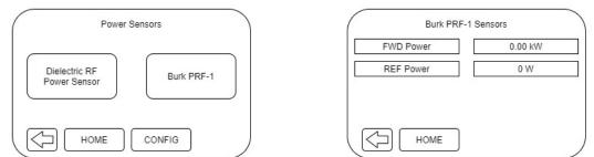
3) Next press REF Power to bring up the calibration screen for the reflected power sensor. The message "Voltage too low" will appear if the voltage sample on the sensor is below 100 mV and not allow calibration of the sensor.
