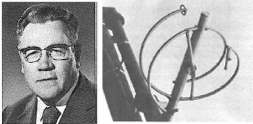
FIGURE 1: MATTI SIUKOLA – RCA’S BFC - FIRST DUAL POLARIZED FM ELEMENT.
