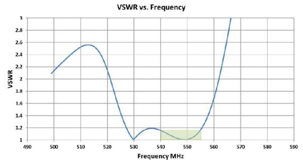
Figure 7: Calculated impedance – VSWR response at points B in Figure 4.
