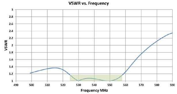
Figure 18: Calculated impedance – VSWR response at points B in Figure 16.
