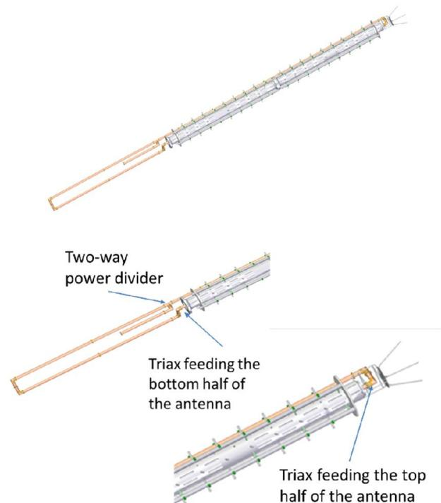
Figure 10: Full antenna design manufactured for Omaha utilizing the phase cancellation scheme shown in Figure 4.
