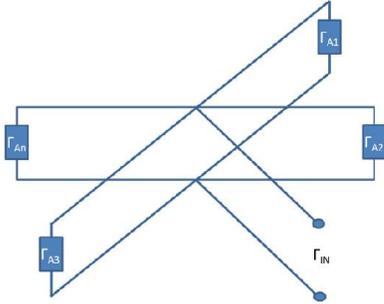
Figure 3: Arbitrary number of loads connected in parallel
