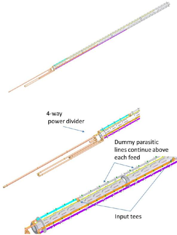
Figure 17: Full antenna design utilizing four tee feeds for the phase cancellation scheme shown in Figure 16.
