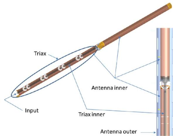
Figure 9: Center feeding a slotted coaxial antenna with layered inner conductors called a triax
