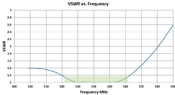
Figure 8: Calculated impedance – VSWR response at points B in Figure 4.
