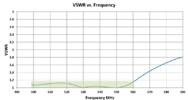
Figure 19: Calculated impedance – VSWR response at point C in Figure 16.
