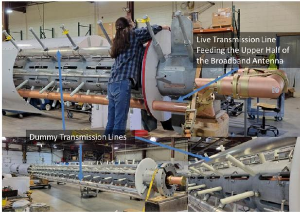
Figure 14: Live and dummy transmission lines placed around the antenna aperture to improve the circularity.
