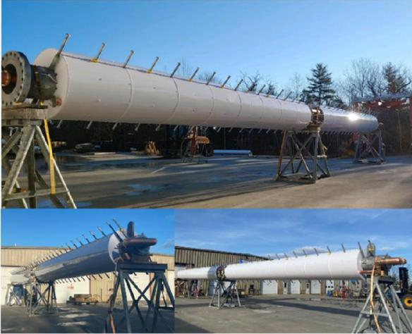
Figure 10: Full antenna design manufactured for Omaha utilizing the phase cancellation scheme shown in Figure 4.
