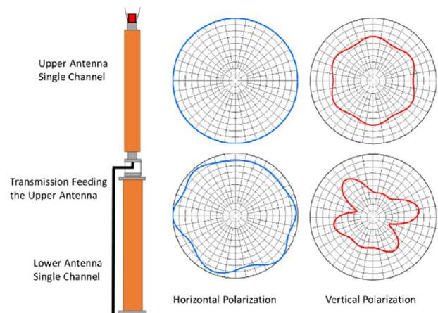
Figure 13: Stacked UHF antenna azimuth patterns. Note the bottom antenna's circularity is affected by the transmission line running up the side of the antenna to feed the upper antenna.
