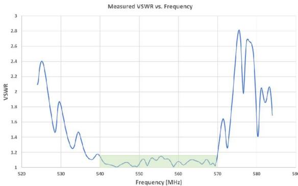
Figure 11: Measured VSWR vs. frequency. Omaha antenna based on phase cancellation scheme shown in Figure 4.
