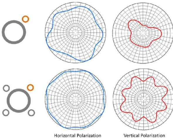
Figure 15: Comparison of the Omaha azimuth patterns with a single transmission line versus the addition of 3 extra dummy lines.
