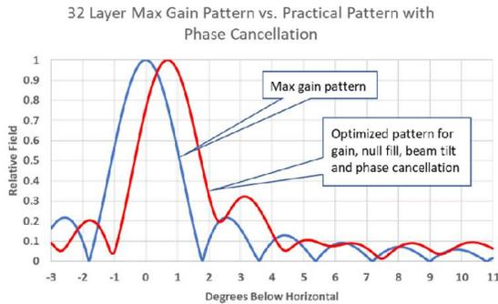
Figure 5: 32 Layer slotted coaxial antenna elevation patterns. Red pattern uses the phase cancellation shown in Figure 4 to increase the operating bandwidth while maintaining .75 degrees of beam tilt, 20% null fill and high gain.
