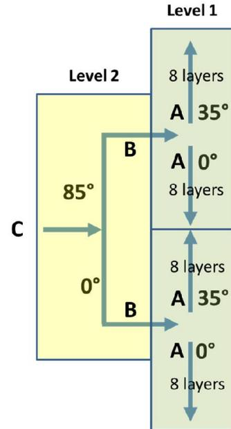
Figure 4: Phase offsets incorporated into a 32 layer coaxial antenna design to provide increased operating bandwidth while maintaining practical elevation pattern parameters.
