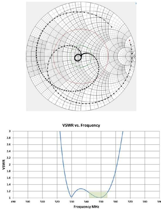
Figure 6: Typical 8 layer slotted coaxial antenna impedance - VSWR response
