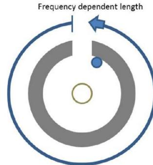
Figure 1: Outer conductor of slotted coaxial antenna creates a frequency dependence causing narrow band operation.
