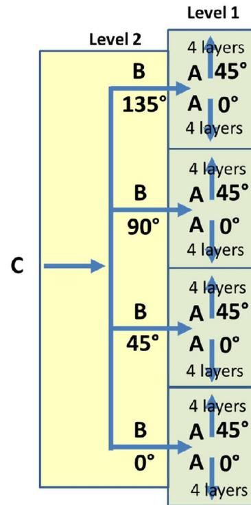
Figure 16: Phase offsets incorporated into a 32 layer coaxial antenna design to provide more operating bandwidth than the scheme shown in Figure 4.
