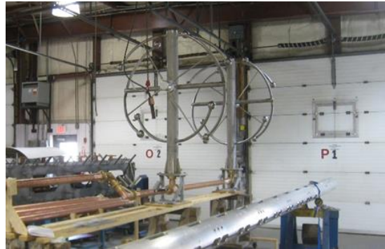
Figure 3: DCR-Q Quadrupole FM style antenna designed and manufactured for channel 3 during Repack.
