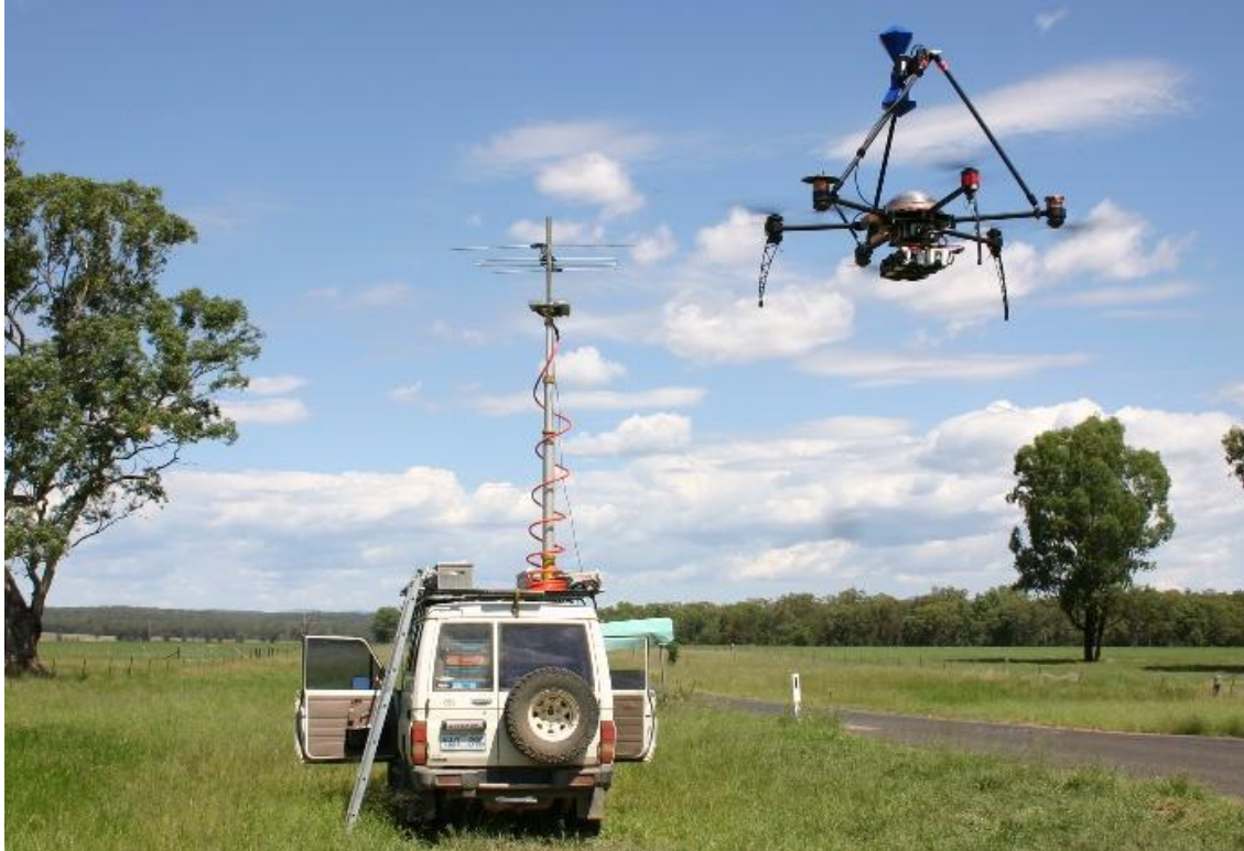
FIGURE 1: FIELD MEASUREMENT TRUCK AND DRONE MEASURING BROADCAST ANTENNA PATTERNS, COURTESY SIXARMS.
