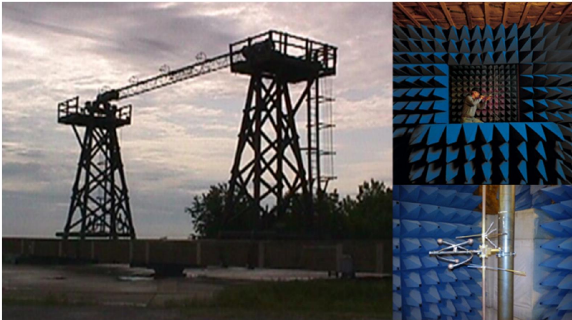
FIGURE 3: LEFT: FAR FIELD RANGE DIELECTRIC / HARRIS, PALMYRA, MO. RIGHT: QUARTER SCALE MODELING IN ANECHOIC CHAMBER – DIELECTRIC, RAYMOND, ME.
