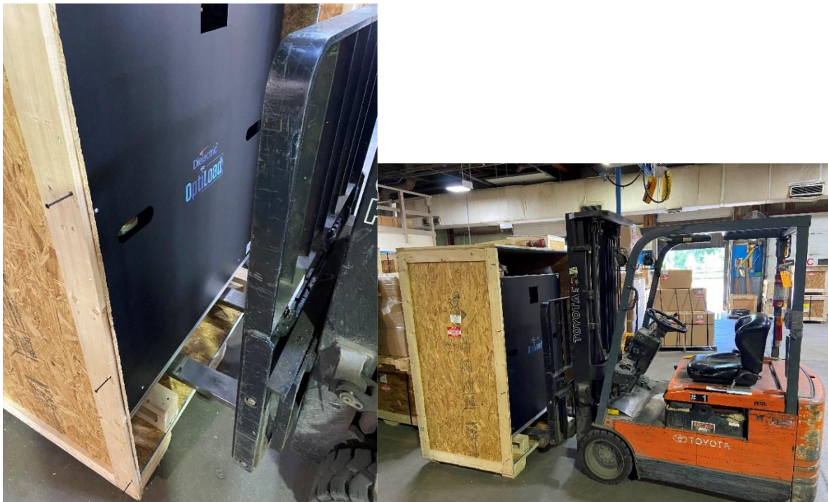
Figure 30: Recommended placement for forks to lift OptiLoad from crate
