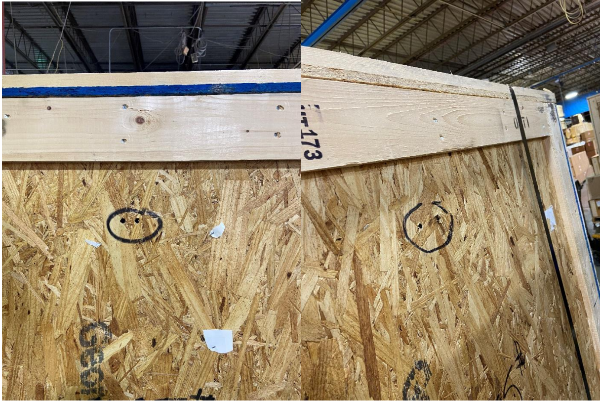
Figure 23: Screws to be removed on the front and rear panels of crate to remove internal cross support Once all these screws are removed, the front panel may drop about 4" to the floor. The panel can be removed to access the unit inside.
