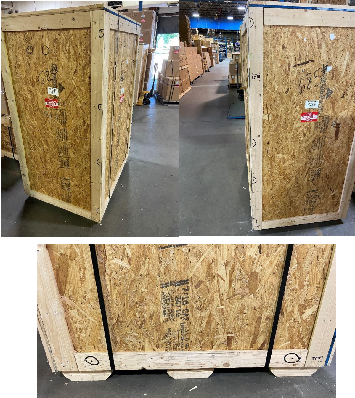
Figure 22: Screws to be removed from the front panel of the crate
