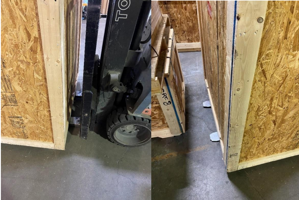
Figure 20: Proper positioning of forks when using a powered forklift
