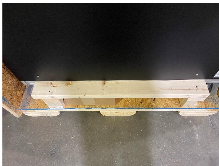
Figure 25: Bottom cleat to be removed
