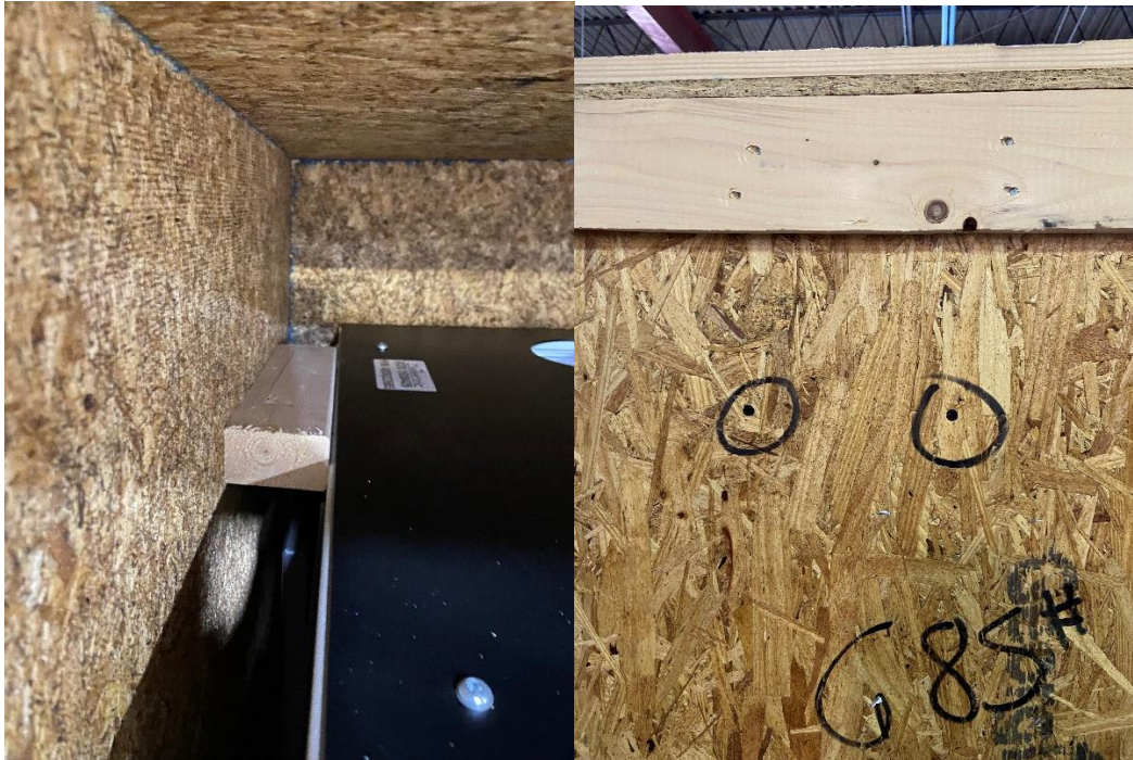
Figure 26: Additional blocking to be removed (on control panel side of crate)
