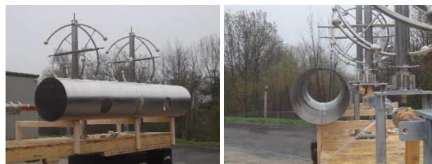
Figure 12: Testing the impedance effect of a large diameter pipe placed close to the helical arms of a broadband ring style antenna.
