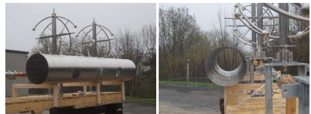
Figure 12: Testing the impedance effect of a large diameter pipe placed close to the helical arms of a broadband ring style antenna.
